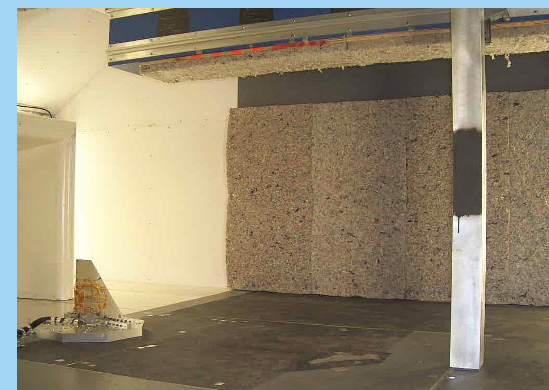
Smart Fin and Tubular Von Karman Vortex Generator in the Wind Tunnel
